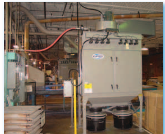
BDC-22T Used to collect fiberglass particulate.
